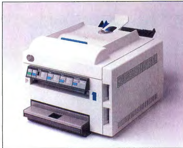
IBM's LaserPrinter features 10 ppm, 300 dpi, and HP PCL emulation; PostScript is promised.
