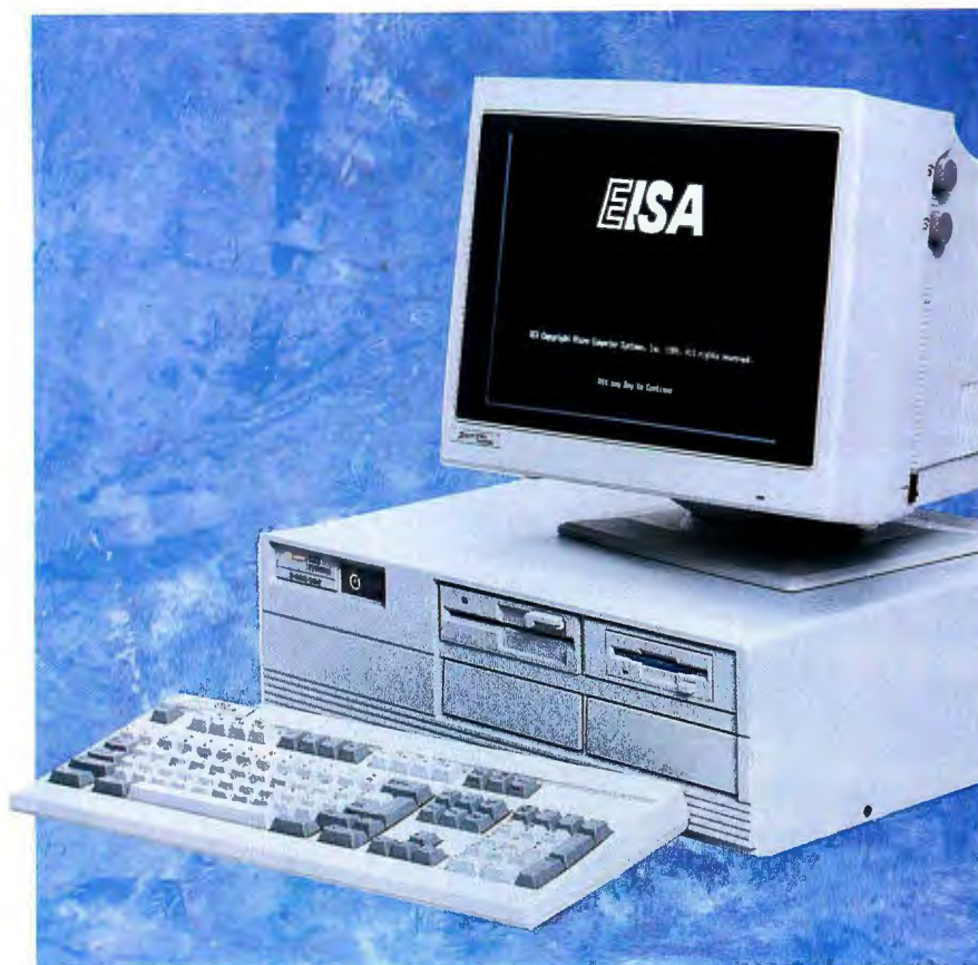
Photo 1: The Zenith Z-386/33E. Except for its EISA slots and disk drive controller, it's virtually identical to the company's non-EISA 33-MHz 80386 system.
