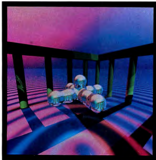
Photo 1: This image, using 16 T414 transputers in a ring, illustrates how ray tracing can reproduce reflections and shadows.
