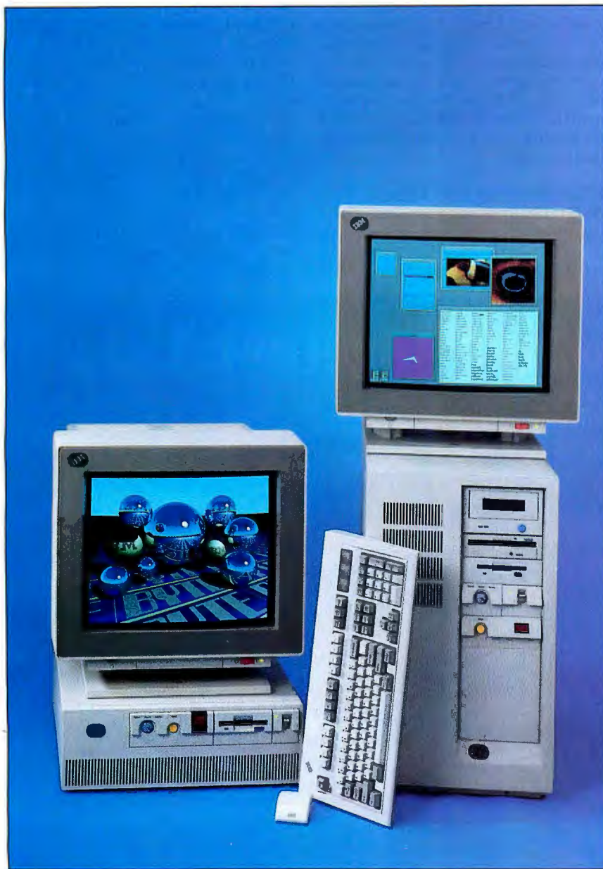
IBM's POWERstation 320 desktop and POWERstation 530 desktide systems. The desktop unit (left) is showing a ray tracing generated by the high-performance three-dimensional graphics board. The desktide system (right) is running OSF/Motif.
