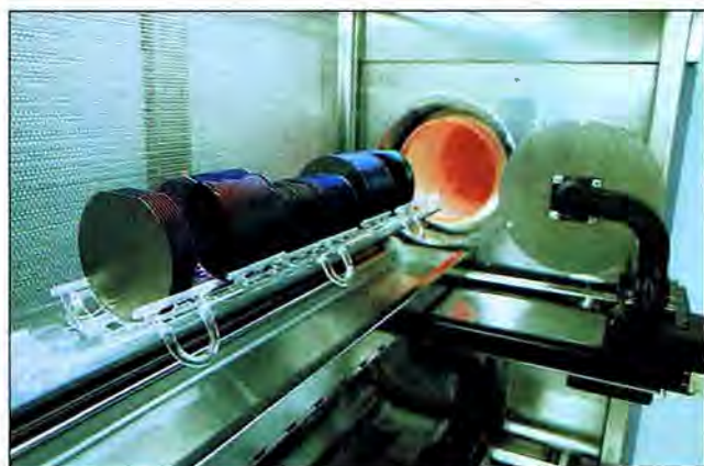
Photo 2: Research at the Austin, Texas, semiconductor consortium, SEMATECH, centers around ways to efficiently fabricate chips. Here, wafers are being prepared for loading into a furnace chamber.
