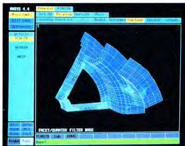
With PC Linear from Swanson Analysis, you can test various types of material before constructing a prototype.
