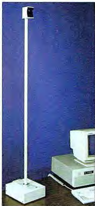
An infrared transceiver from Untied TeleCom connects you with Ethernets and Token Rings.
