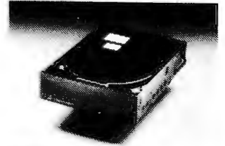
5-1/4" Half-Height Rigid Disk Drive
