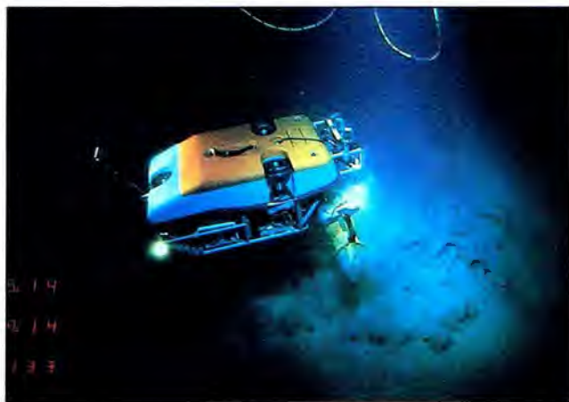
In 1989, Jason surveyed and excavated a fourth-century trading vessel lying 700 meters deep in the Mediterranean sea. Here the vehicle employs a specially designed robot arm to recover an amphora, or large vase, from the wreck. (Photo courtesy Quest Group, Ltd., and Woods Hole Oceanographic Institution)
