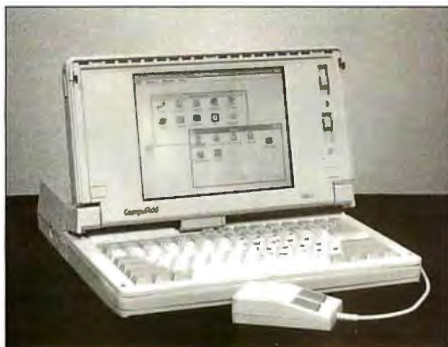
The CompuAdd 316SL uses 12-V and nickel-cadmium batteries and ships with power-management software. The 316SL weighs 11 1/2 pounds.
