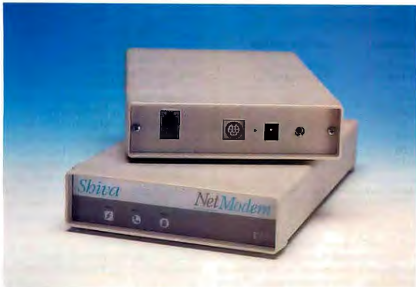
Shiva's NetModem V.32 offers 9600-bps communications as a shared network device or as an internetwork router, thanks to its built-in AppleTalk connector (top).
