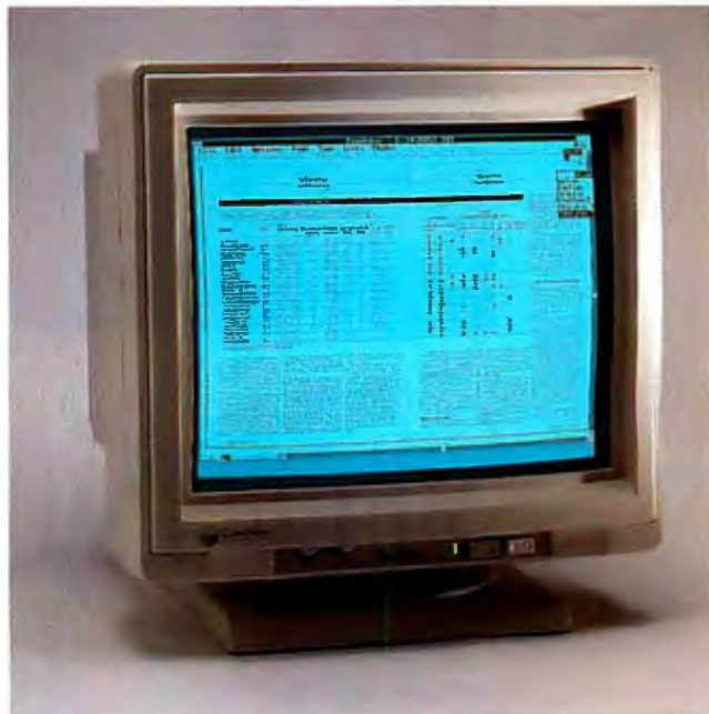
Cornerstone's DualPage PC offers 1600- by 1280-pixel resolution and an upgrade path to 4 or 16 gray scales.
