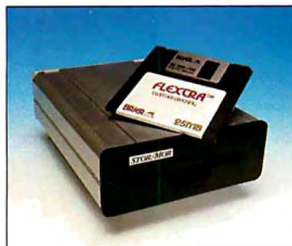
The Stor/Mor Subsystem uses a SCSI controller to bring 20-MB floppy disk storage capacity to PCs and PS/2s.
