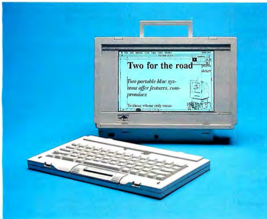
The Outbound performs comparably to the Mac Portable, but it needs the ROMs from your Mac Plus or SE to operate. Note the IsoPoint pointing device below the space bar.
