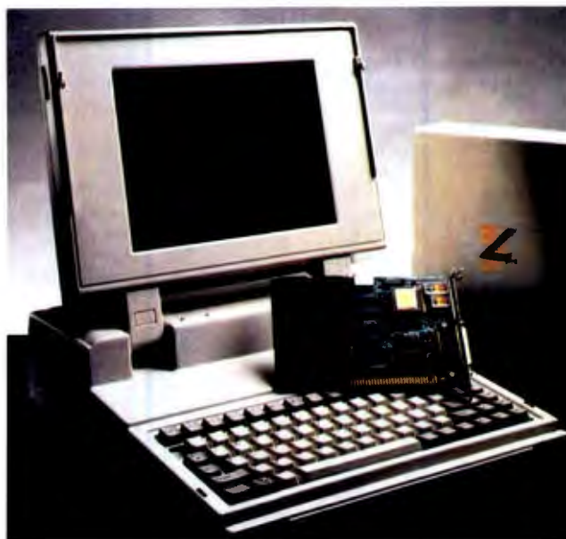
Paratech Solutions' PST360X Jet Series laptops combine the flexibility and convenience of a laptop with the power of a 20- or 30-MHz 32-bit T800 or T805 transputer with 4, 8, or 16 MB of zero-wait-state DRAM.
