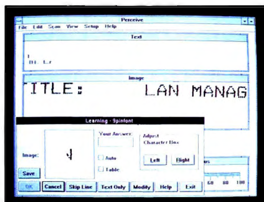
Screen 2: Because dot-matrix characters are made up of a series of dots, many OCR packages detect the individual dots and interpret them as dashes, periods, or apostrophes. Sometimes, as shown here, only part of a character is read. Perceive's learning facility includes a Character Box, which you can adjust to account for misreads.
