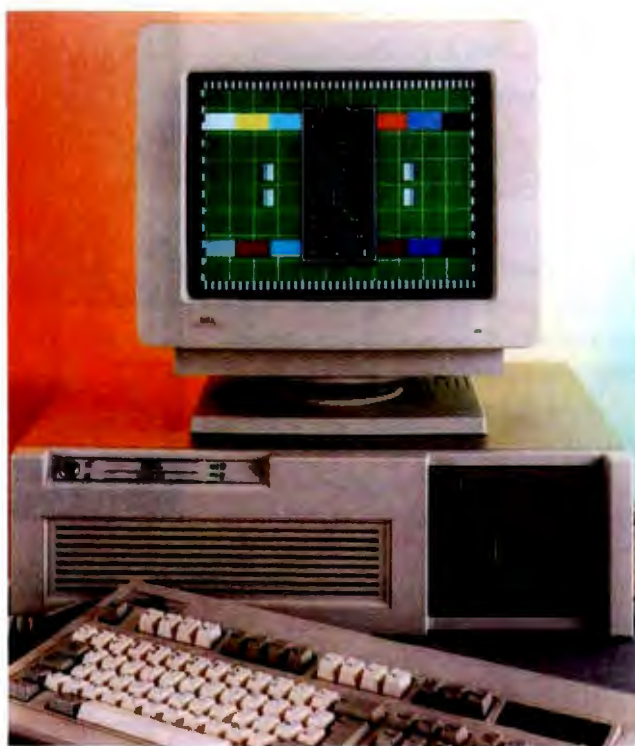
TestCard software lets you analyze the performance of your monitor using the patterns and colors that professional service engineers use.
