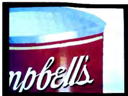
Photo 2: The can top was created by first drawing an ellipse, which was then reshaped using a perspective tool and filled with graded shading.
