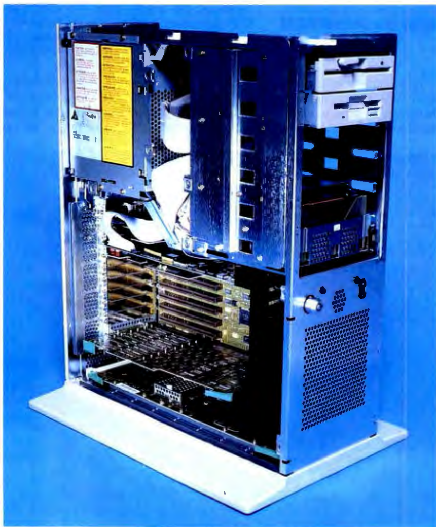
The HP Vectra 486/33T is solidly designed for full-time heavy-duty use and EISA expandability. The processor is located on its own daughterboard.
