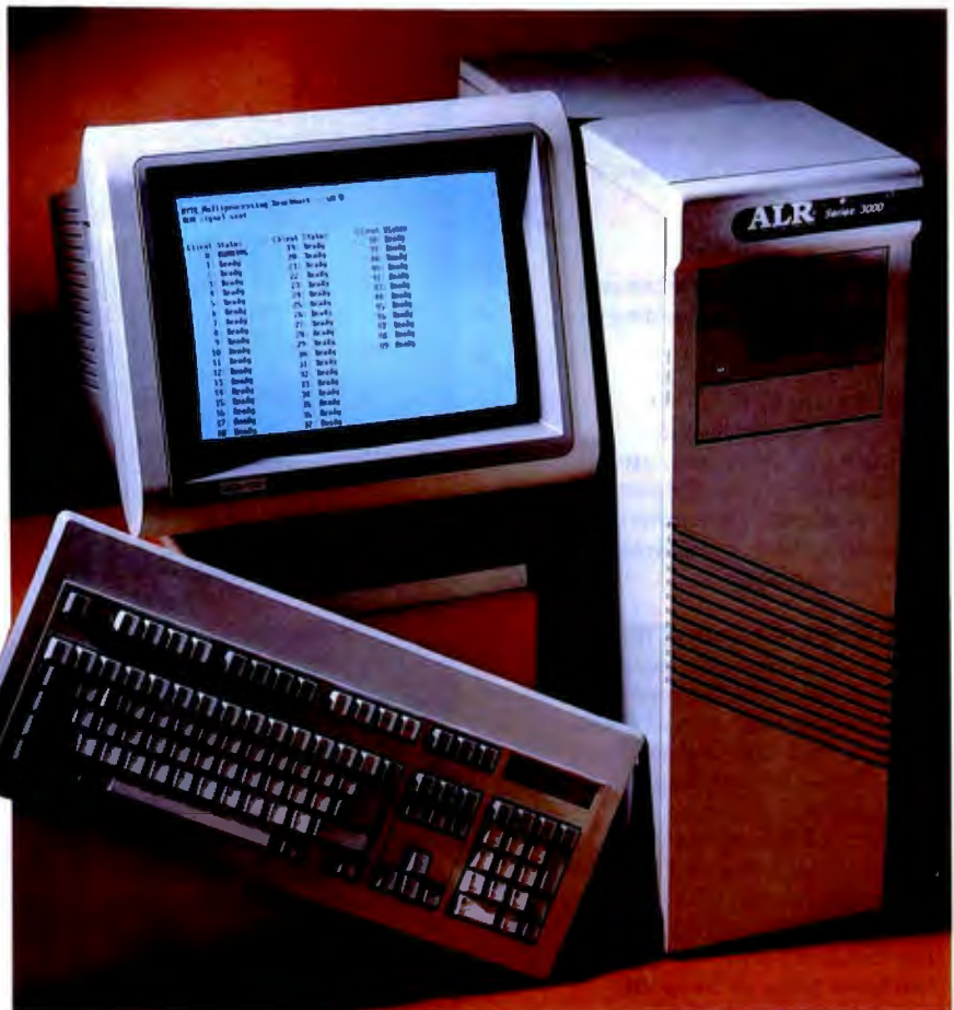
Photo 1: The MultiAccess Series 3000 symmetric multiprocessing system holds up to six i486 processor boards. SCO Unix and the MPX multiprocessing kernel coordinate processor activity.
