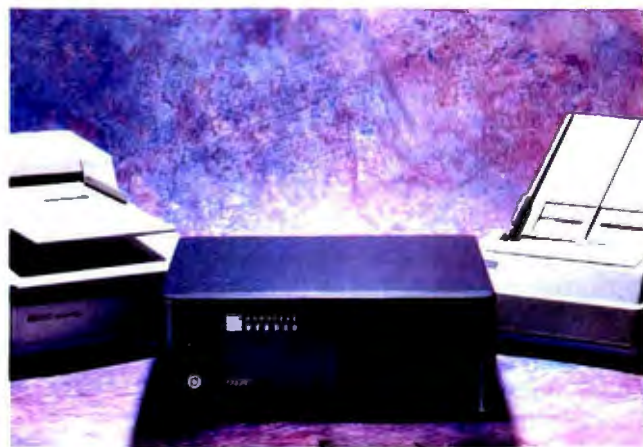
Photo 1: The Parallel Reader, which packs four 68020 processors working in parallel, supports the Hewlett-Packard ScanJet Plus (shown at left with optional document feeder), the Microtek MS-II (right), and the Fujitsu 3093 (not shown).
