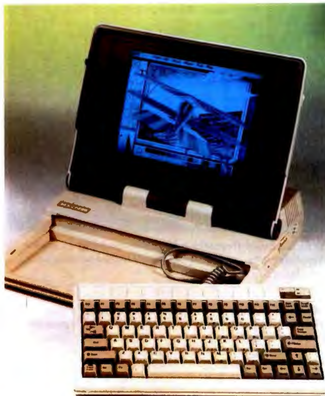
Diode Export's DEX-CP286 laptop has an 80-key detachable keyboard with 12 function keys and a coil cable.
