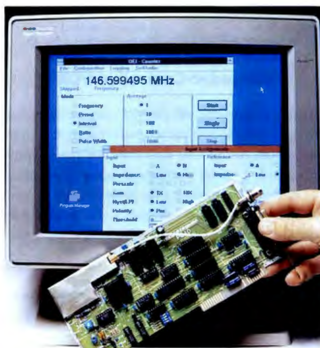
Optoelectronics' PC-10 Universal Frequency Counter uses Windows 3.0 for instrument control.
