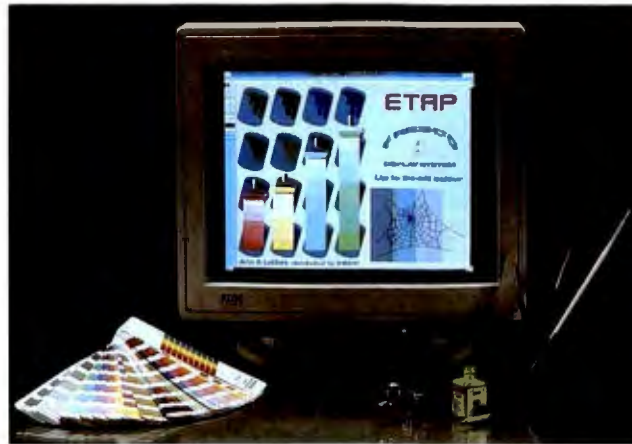
The Fresco 2 dual-frequency color monitor provides 8-bit color in resolutions of up to 1280 by 960 pixels and 24-bit color at a resolution of 512 by 384 pixels.
