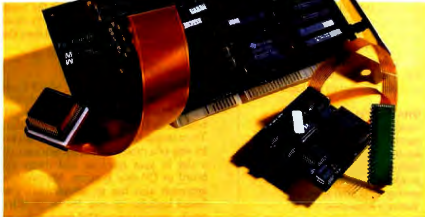
The FastCache-SX upgrade board (left) fits into a 16-bit ISA slot and connects to an AT system's 286 socket by way of a special plug and cable. The Cumulus 386SX card (right) plugs directly into the 286 CPU socket. Both accept an 80387SX FPU.
