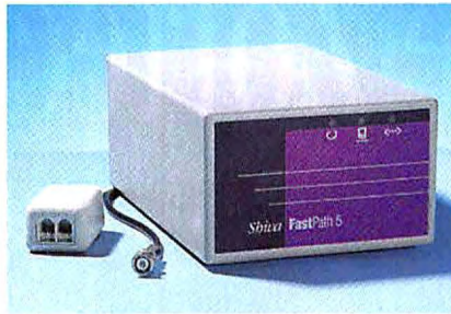
Photo 1: Shiva's FastPath 5 LocalTalk-to-Ethernet gateway supports AppleTalk Phase 1 and 2, TCP/IP, and DECnet Level 1 protocols. Rather than implementing an NFS gateway within the FastPath, Shiva bundles a copy of InterCon's NFS/Share NFS client, which runs on each Mac.
