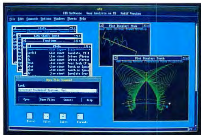
TK Solver for Motif running a gear analysis, showing functions, plots, and charts simultaneously.
