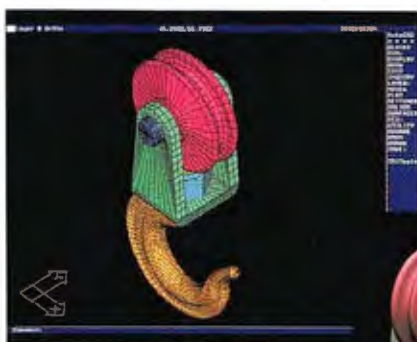
Screen 2: The block-and-tackle model using Silicon Graphics' IrisVision adapter and ADI driver. (Top) The wireframe image has AutoShade flat shading applied while inside AutoCAD. (Right) The model was exported as a DXF, and then, after exiting AutoCAD, Gouraud shading was performed using IrisView, Silicon Graphics' real-time animation and walk-through software.
