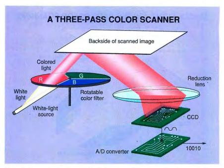
Figure 2: For each scan line, a white-light source shines through red, green, and blue filters.
