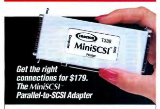
Add a SCSI port to almost any printer port with our pocket-sized, self-contained MiniSCSI. Ideal for laptops, notebooks and systems which can't accommodate a standard SCSI interface, the MiniSCSI also lets you relocate SCSI devices easily.
