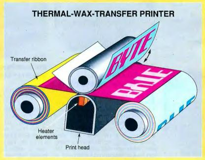
All thermal-wax-transfer printers work by heating colored wax (cyan, magenta, yellow, and black) and fusing it to a special paper. The print head melts tiny dots of color from a ribbon onto the paper. The paper must make four passes by the ribbon and heating element—one pass for each of the four colors.
