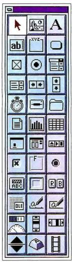
The Toolbox provides instant access to 36 controls.
