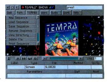
athematica's Tempra Show is a DOS (not a Windows) program that has a GUI wrapper. Presentations created with Show can be played back on any properly equipped DOS machine (a PC with at least a 286 processor, 540 KB of main memory, and 5.5 MB of disk space). This is a very capable but easy-to-use presentation package, and I like its results.
