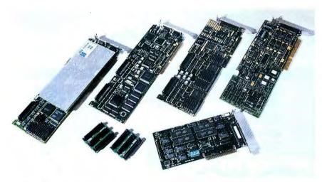
Studio's hardware consists of five boards (four ISA and one EISA). The first three (working from left to right) handle video, and they communicate with each other via a set of bus sockets along the top of the boards. The fourth is the DSP-based audio processing board. The smaller board below the others is the four-port RS-422 VCR controller.
