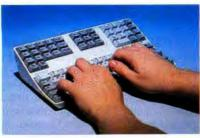
First successful alternative to conventional keyboard saves 60% desk space with a foot print of 27.3 x 15.2 cm. Has full travel tactilly responsive keys with standard left-right spacing for easy touch typing. 100 keys, compatible with IBM XT/AT PS/2. Many language versions available.
