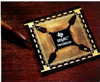
In addition to breaking price barriers, the highly integrated microSparc chip consumes much less power than comparable SPARC processors, making it ideal for portable computers.
