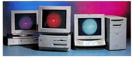
Although housed in Centris/Quadra-type cases, the new Power Macs provide RISC performance at affordable prices. From left to right: the 6100/60 with 60-MHz PowerPC 601 CPU, the 7100/66 with 66-MHz CPU, and the 8100/80 with 80-MHz CPU. Prices start at \$1819 for the Power Mac 6100/60, with 8 MB of RAM and a 160-MB hard drive but without a monitor or keyboard.
