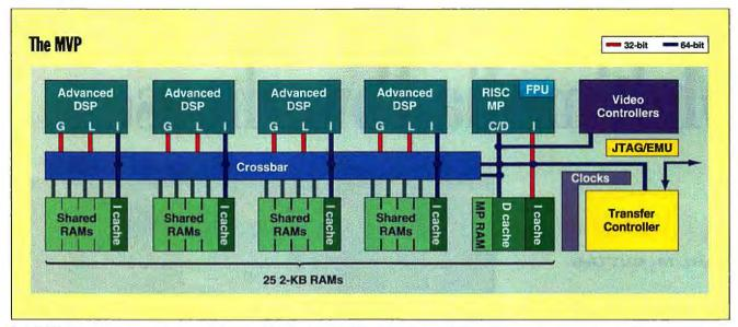
Each ADSP has two independent 32-bit data ports (G and L in the figure) and a 64-bit instruction cache input (I). The MP has a single 64-bit data port (C/D) and a 32-bit instruction port. The TC (Transfer Controller) has a 64-bit internal port and a 64-bit external port. The ports of the various processors and TC are connected to 25 2-KB RAMs via a crossbar-switch network. The crossbar supports approximately 2.4 GBps of data, plus 1.8 GBps of instructions.
