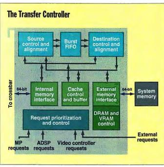
In addition to controlling the movement of data and instructions on- and off-chip, the TC performs transformations where data is processed in an order different from that in which it is stored. The TC also contains a DRAM and VRAM controller.
