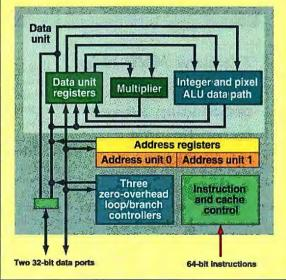
Like other DSPs, those integrated with the MVP are built to support multiple data accesses in a single cycle and to optimize the performance of the multiply-accumulate operations that characterize signal-processing algorithms. In addition, the ADSPs also support bit-field and pixel operations, making them powerful imaging and graphics processors as well.
