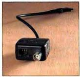
used is auto-selectable. The 3Com EtherLink III offers a similarly flexible design. It comes with two types of cables, one with a BNC connector and the other with a twisted-pair connector.
