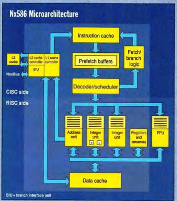
The Nx586 combines a CISC front end with a RISC-like processing core. It employs dynamic branch prediction and speculative execution to keep its deep pipelines busy.
