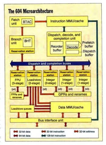
cations. Registers and memory can be touched only by nonspeculative instructions in program order. This rule is enforced by the completion unit. (The exceptions to this rule are the Counter and Link registers used by branch instructions. These employ shadow registers to back out of mispredicted branches.)
