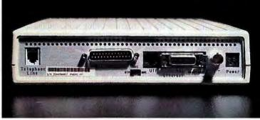
The NetBlazer PN1 provides all three types of Ethernet connection (AUI for thick coaxial cable, BNC for thin coaxial cable, and RI-45 for twisted-pair cable), a phone connection for its internal V.32bis modem, and a 25-pin serial port for attaching a second modem.
