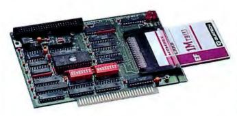
The PCMCIA standard allows the information gathered via laptop, PDA, palmtop, or pen-based systems to be compatible with desktop PC's. Quatech manufactures a full line of products that conform to the PCMCIA standards including Type I card readers for memory cards, Type II and III interface adapters, and I/O cards for communications and data acquisition applications.
