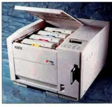
The Xerox 4900, showing its color toner cartridges and internal floppy drive.
