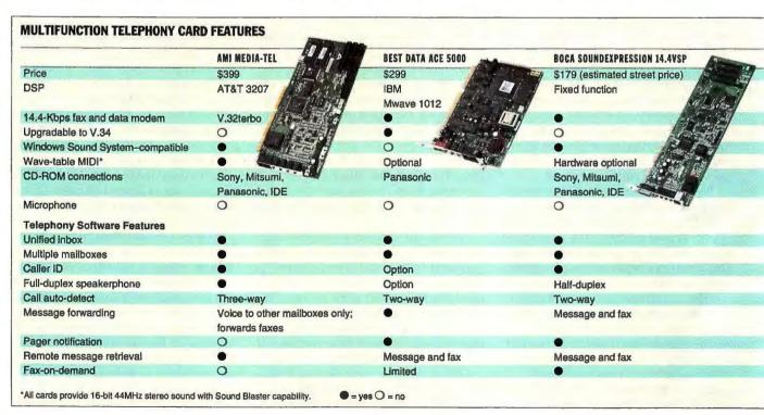
length card uses IBM's MDSP1012 Mwave chip, and its features and DSP software capabilities are similar. A joystick/MIDI connector is standard (through an adjacent slot opening), and the audio connections (microphone, line in and out) run through a pigtail. There is a bundled microphone, and the card has a scanner port and software that supports scan to fax, giving you real fax-machine capability.
