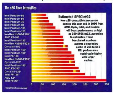
A 180-MHz Pentium would likely break the 200-SPECint92 barrier and deliver roughly the same performance as the first P6, which is clocked at 133 MHz. By then, of course, the P6 will be faster, too. Intel plans to introduce a 166-MHz P6 in early 1996 and a 231-MHz version later next year. That would yield an estimated top end of about 350 SPECint92, which would boost the P6 into the stratosphere of the fastest RISC chips.
