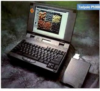
ing to place the floppy drive atop the power brick—bad move. Electromagnetic fields from the power brick made the floppy drive unreliable for reads and writes. Disk reads were agonizingly slow, and formatting a blank floppy disk was impossible. The interference doesn't appear to cause any permanent damage, however. Separating the power supply and the floppy drive as much as their cords allow returned the floppy drive to normal operation.
