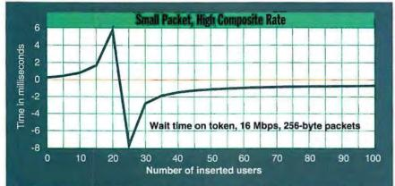
This illustrates a 512-Kbps throughput demand that a composite set of nodes places on the network. The 256-byte packets are uniform but small, and the waiting time for a token builds to roughly 6 ms before going negative at approximately 20 inserted stations. At that point, the real-world network becomes unstable and can drop packets.
