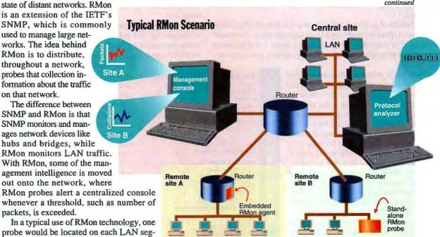
RMon probes distributed throughout a network collect traffic information that is called up on a central management station. Protocol analyzers are then attached to a LAN it easy for a manager at a central site to analyze segment when more detailed packet analysis is needed.
