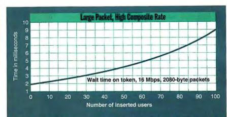
Here data-transfer efficiency increases, because far fewer transmissions are required to move the same volume of data. Therefore, the network is stable right up through 100 inserted stations. However, once we get to 50 stations, the wait time begins to exceed the transmission time.
