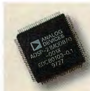
Analog Devices' ADSP-21mod870 (actual size) puts the functionality of a modem on a single chip.
