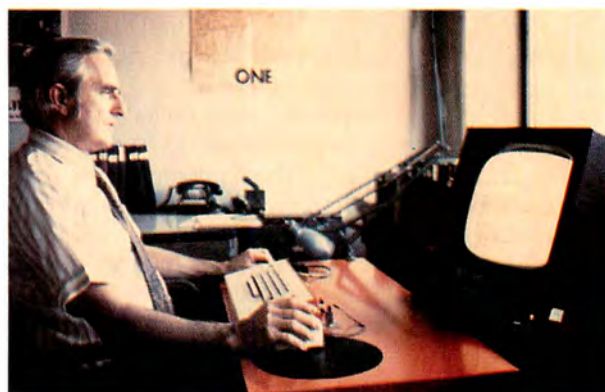
Figure 6 Engelbart operating a prototype of the NLS system developed by his team at the Stanford Research Institute. He enters letters, numbers, and symbols with his left hand via a five-fingered chord keyset while his right hand manipulates a cursor with a mouse.
