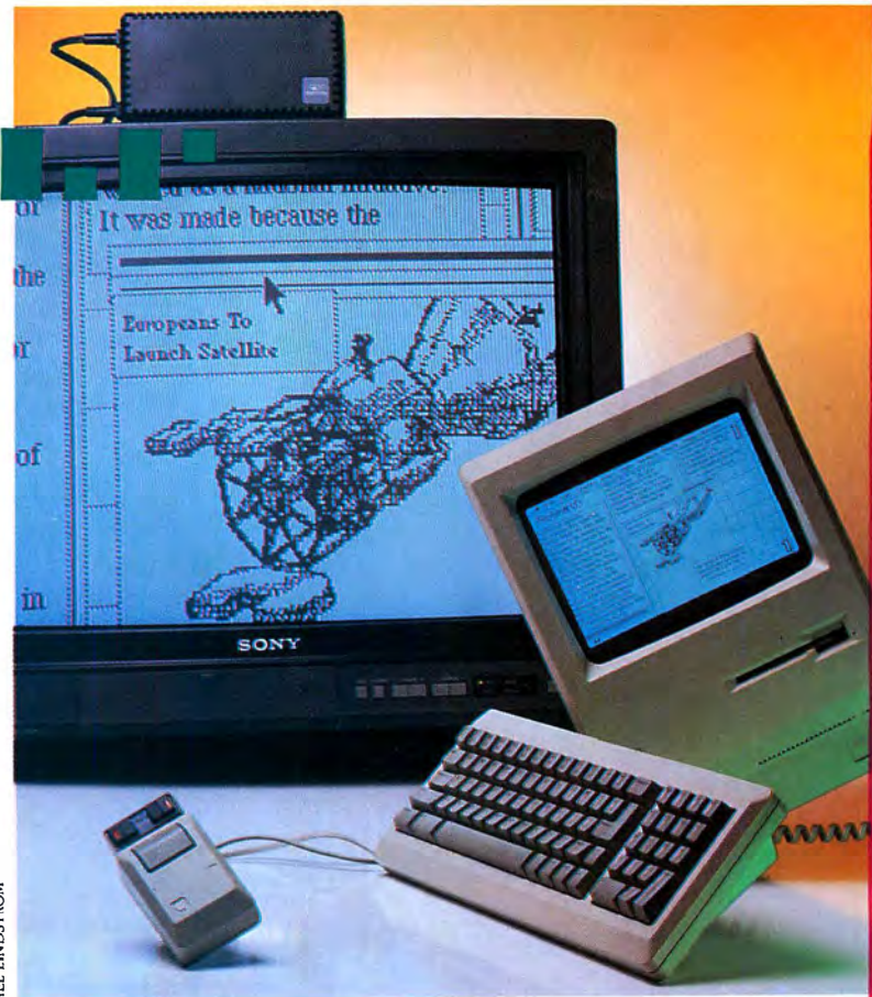
The MacVideo Processor, which is installed on the back of the Macintosh, displays enlarged Mac images on standard TV screens.
