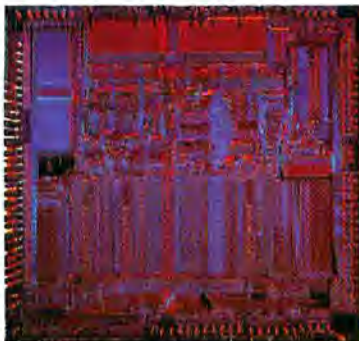
The heart of the new Mac—the Motorola 68020 chip.
