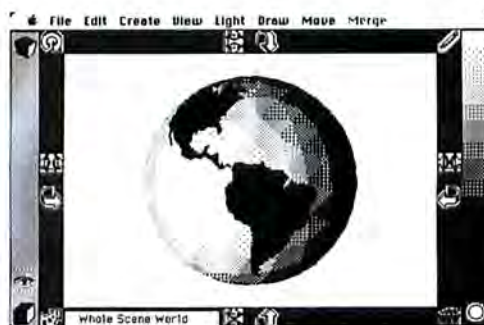
Figure 2 Easy3D can be an efficient animation tool. Move a 3-D object by degrees and save your changes as a series of MacPaint documents. The program also lets you adjust lighting and select a background shade.
