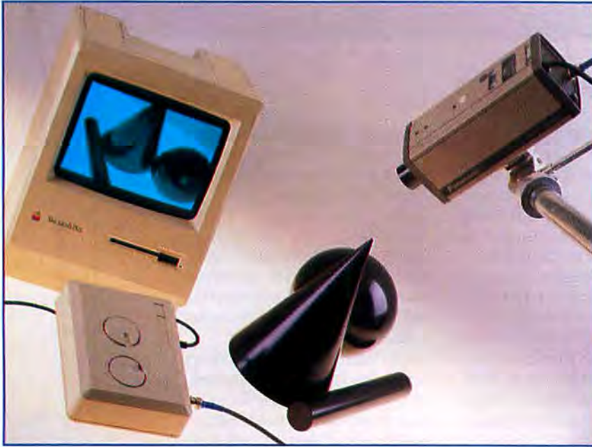
Figure 2 Portable cameras with multiple-pin connectors cannot attach directly to the MacVision digitizer. You can use a videocassette recorder as a power supply and signal source by connecting the camera cable to it. Route a video cable from the video-out terminal on the VCR to the video input of MacVision.
