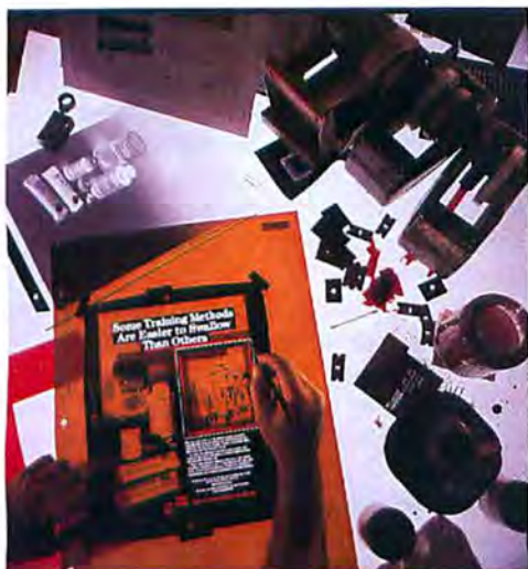
A stripper uses Rubylith and orange tape to block out all but the desired elements for the black layer of a four-color ad. This negative will then be transferred to another negative, which will be used to create a printing plate.
