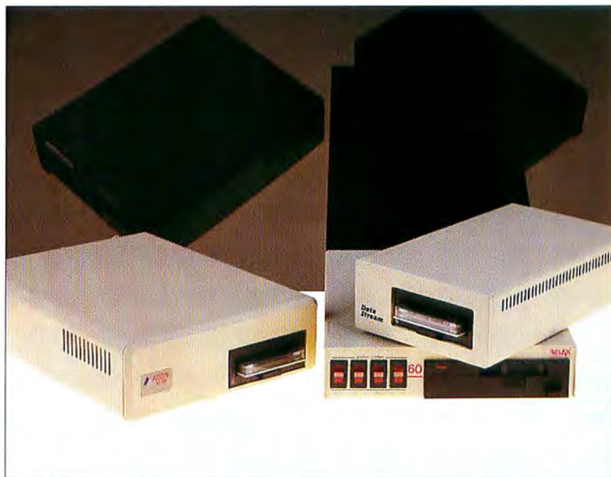
Both Adon's TD-40 (left) and SuperMac's DataStream (top right), like Apple's drive, use the DC 2000 cartridge. Relax's Tape 60 Plus uses a digital cassette.
