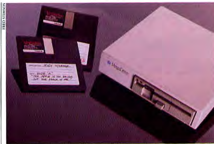
The MegaDrive's 5¼-inch floppy disks offer portability at near-hard-disk speeds and capacities. Data on the 10MB floppies last ten times longer than on Bernoulli-technology cartridges.
