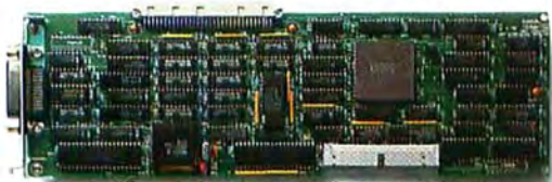
In scientific or engineering applications, a special card can connect an SE or a II to lab instruments.
