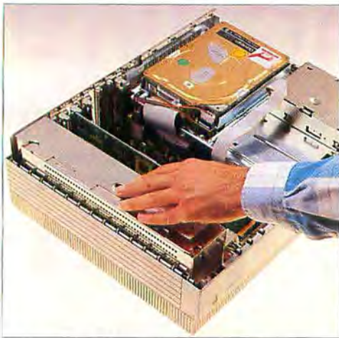
Step 5: Touch the power supply to discharge static electricity.
