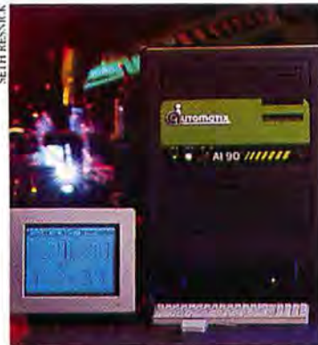
This hardened cover hides an industrial-strength Mac II ready for tough conditions.
