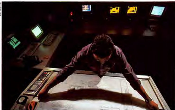
Rolling out of this electrostatic printer, which is much faster than a plotter, comes a 44-inch-wide blueprint at 400 dpi.
