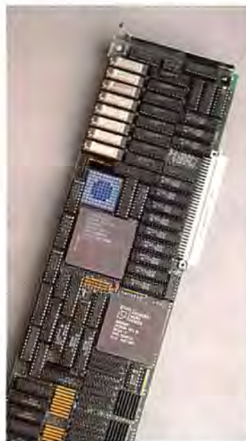
A Mac II with YARC's McCray board can compute 20 times faster than a Mac II with the 68881 math chip.
