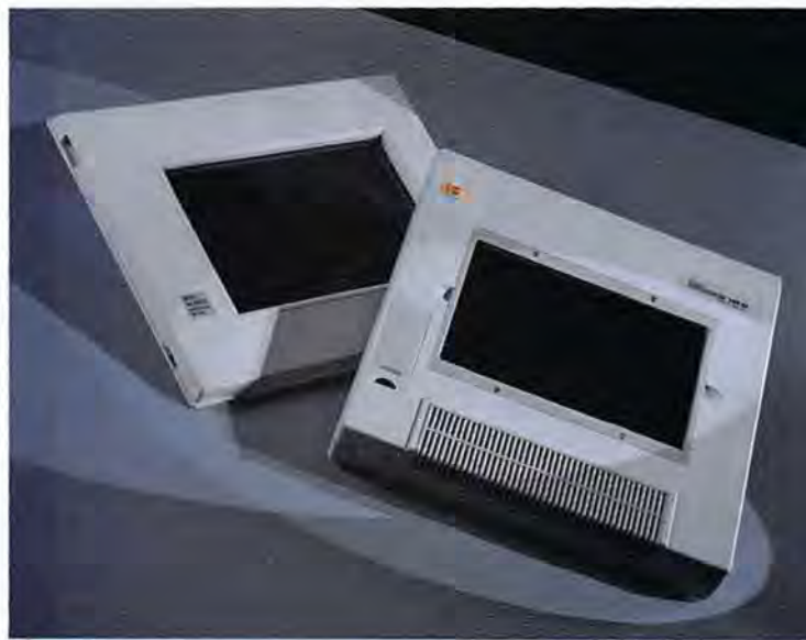
The Ask Mac-Screen Overhead (on the left) has a viewing size of 8.3 inches by 5.6 inches and weighs 3.2 pounds. The Kodak Datasbow's viewing size is 6.5 inches by 4.4 inches, and the unit weighs 6.6 pounds.
