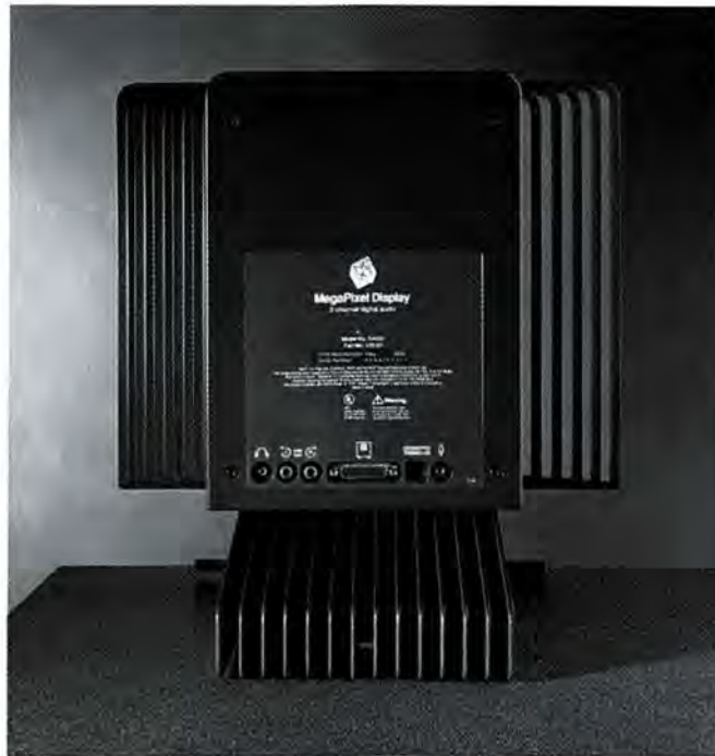
The back of the Mega-Pixel Display, showing (left to right): the stereo headphone output; standard RCA stereo line-out ports; connector for cable from Next computer; standard microphone input.
