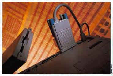
Rapport plugs into a Mac 512KE, Plus, or SE and lets you read files from, and write files to, 31/2-inch IBM disks.
