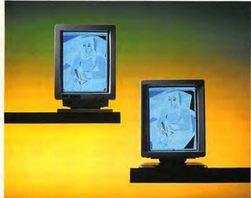
video board gives it a slightly lower resolution of 1024 by 768. The display is clear and crisp, with no visible bowing or other distortion along the edges. There is some ever-so-slight blurring along the right edge, and the display is slightly off-center horizontally (toward the right), but these are very minor faults.
