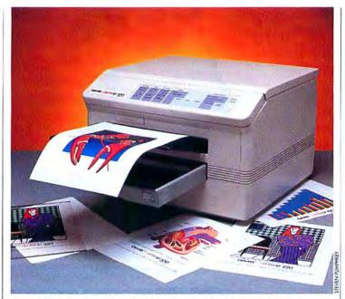
The QMS ColorScript 100 Model 10, the first 300-dpi PostScript printer to cost under \$10,000, is a thermal-transfer device.
