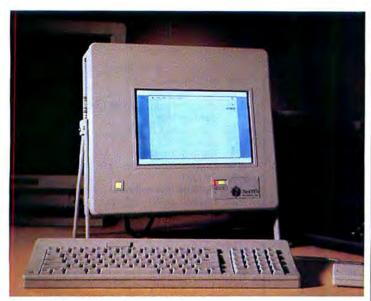
NexSys's Travel Mac fits under an airline seat and uses an easel to adjust the position of its LCD screen.
