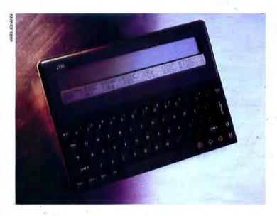
MacLite, the batterypowered Sinclair Z88 from Cambridge North America, weighs less than 2 pounds.
