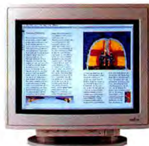
The Radius Color Display showing two full pages. (1152 x 882 pixels)
