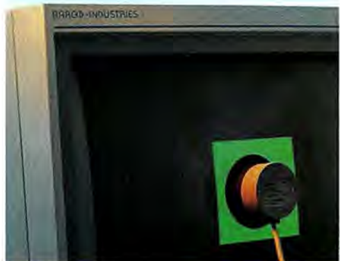
Barco's Calibrator is a combination of intelligent monitor, optical sensor, and color-calibration software.
