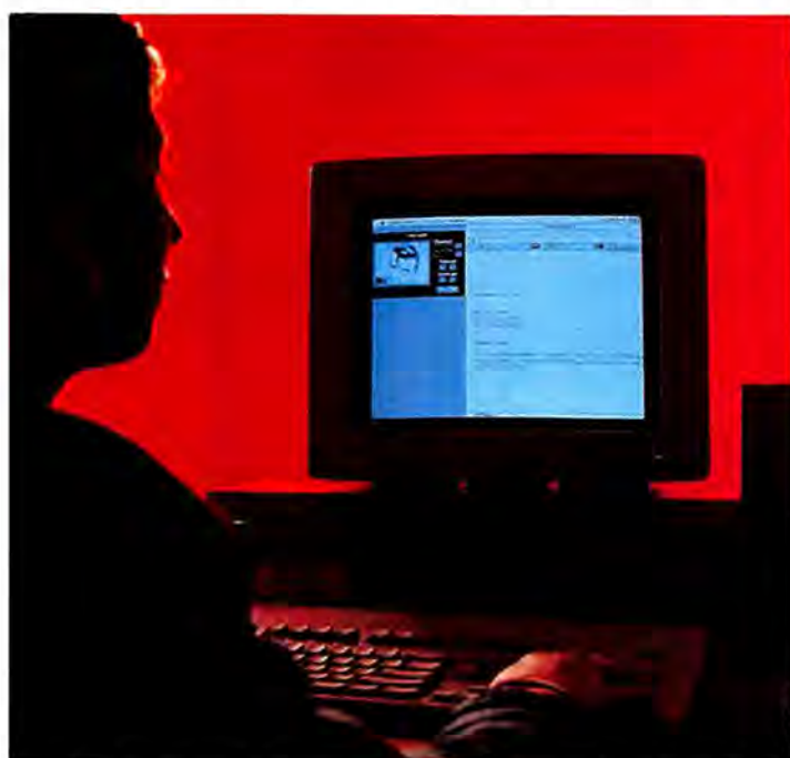
MicroTV from Aapps displays a small black-and-white TV picture (upper left of monitor screen).
