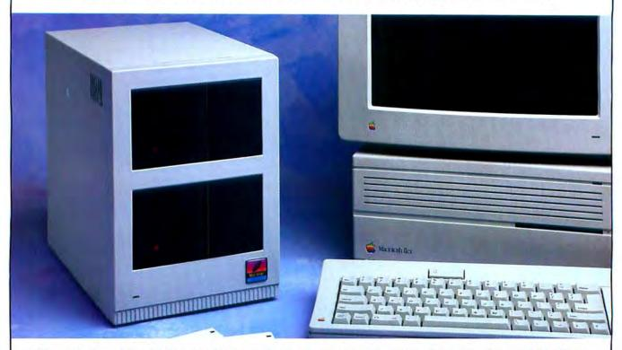
Micro/Spliced Rapid Access Storage Systems are excellent for disk intensive applications, such as, sound, desktop presentation, file servers, CAD and computer-aided-publishing systems. These subsystems seek half as far, half as often and increase transfers up to 60%.
