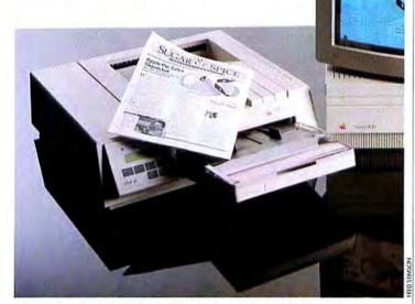
GCC Technologies' PLP II page printer uses an LED array to produce 300-by-300-dpi output.
