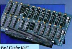
The high-performance cache card for Apple's new Mac Ilci. This powerful new cache memory board plugs directly into the Mac Ilci's cache connector. Fast Cache Ilci boosts processing speed
