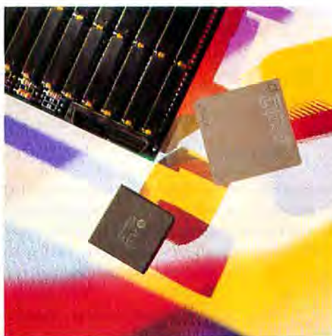
Three different approaches to 24-bit color accelerators: clockwise, from the top, are shown SuperMac's VLSI chip set, RasterOps' AMD processor, and Radius's Acorn chip.
