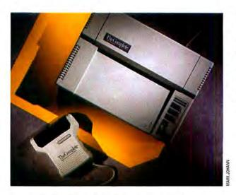
The Complete Half-Page Scanner/400 (left) has a third roller that makes straight scanning easy. The Complete Page Scanner (right) produces crisp, highquality scans.
