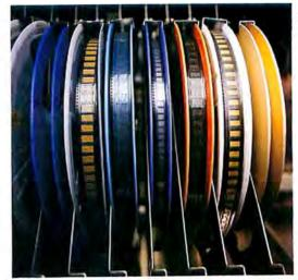
THE JOURNEY BEGINS The Mac's journey really starts here, with the chips that make up a circuit board. These chips come in strips that are wound around plastic 35mm (or larger) reels. Shown here are resistor packs (square, yellow chips), logic arrays (square, black chips), and oscillators (square, metallic chips). Once employees place these reels into automatic parts insertion machines, the factory spins into motion.
