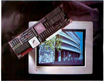
The YARC NuSuper coprocessor board includes a RISC microprocessor that accelerates CAD/CAM performance on the Mac II series.
