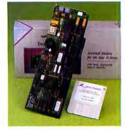
A new internal modem for the Mac II series. Comes with software and a "Mac standard" serial port. Can be upgraded to include MNP error correction. A fax option is also available.
