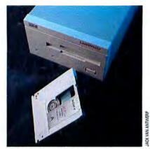
Tecmar's LaserVault 650 erasable optical drive stores 650MB and can work with Mac, PC AT, and PS/2 systems.
