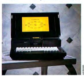
The Dynamac SE/30 comes with an Apple SE/30 logic board and an internal fax modem installed.
