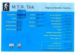
A FileMaker Professional database layout showing radio buttons and buttons that launch actions such as printing.
