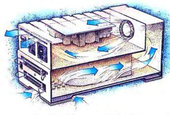
Heat is usually the cause of hard drive failure. We've designed the Protegé hard drive to draw dangerous heat away from the drive assembly and power supply - the two most important components of your hard drive. The fan draws air around the drive itself and then blows the air past the power supply, forcing heat out of the vents and cutting the danger of heat-related failure.
