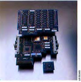
On the DayStar PowerCards, one board (top) contains banks of SRAM. The main accelerator board (middle) holds the SRAM board, the faster processor, and the math coprocessor.
