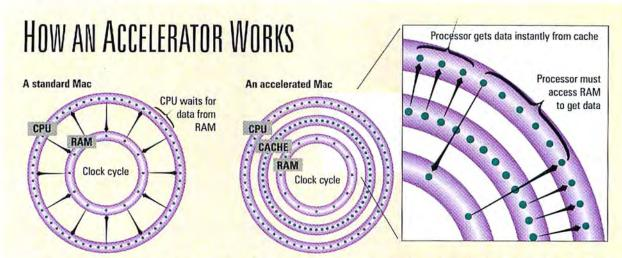
In a standard Macintosh, the processor must fetch instructions from the RAM where they are stored. But because the Mac's RAM is slower than the processor, the processor must wait to receive the instructions. The processor is ready to work at each point in the diagram where there is a green dot. But processing can be done only when the data in RAM is synchronized with the processor (which is displayed here with arrows).
