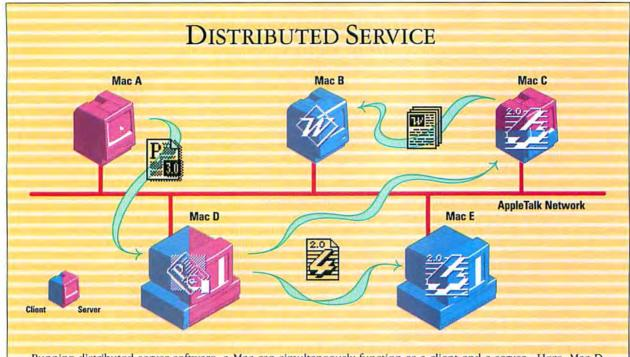
Running distributed server software, a Mac can simultaneously function as a client and a server. Here, Mac D (running PageMaker) is a client of Mac A. Mac D is also acting as a server to both Mac E and Mac C (both running 4th Dimension, a multiuser application). If the distributed server supports multiuser access, Mac E and Mac C can actually be accessing the same 4D file on Mac D. Mac C is also a server for Mac B (running Microsoft Word).
