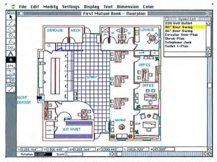
Adding a swinging door to a floor plan from Generic CADD Level 3's integrated object library. Data can be entered directly into the parameter boxes along the bottom.
