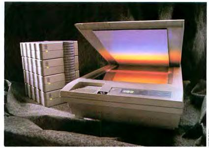
La Cie's Tsunami series of external hard drives (left) stores from 20MB to 210MB. The company's Silverscanner (right) scans in 24-bit color or in 256 shades of gray.
