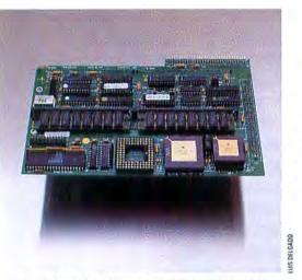
Even though Total Systems' Gemini board contains all of its hardware on one board, it is harder to install than the DayStar PowerCard, the Siclone Si3033, or the Total Systems Voyager. You need a Killy clip to strong-arm the Mac's original processor into a slot on the board.
