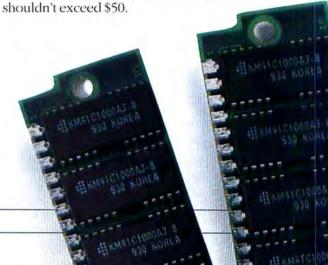
The Mac Plus and Mac SE have four available slots on the motherboard, which originally contain four 256K SIMMs modules - totalling 1 megabyte (1MB) of memory. To upgrade, you can replace each 256K module with a 1MB module, but you must do this in pairs.
