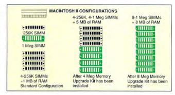
The Mac II, IIx, IIcx and SE/30 each come with a total of eight slots. The standard configuration has four 256K SIMMs modules, or a total of 1MB. Here, memory must be upgraded in multiples of four. This allows for expansion from 1MB to 4MB, 5MB or 8MB.
