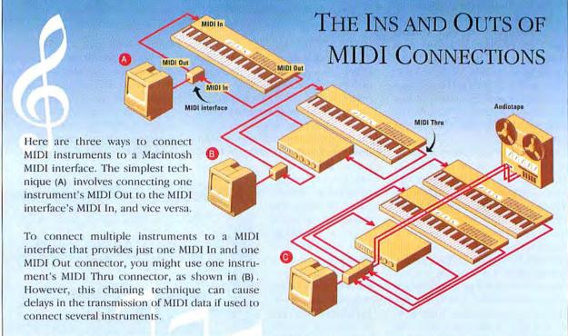
For advanced MIDI setups such as the one shown in (C), it's better to use a MIDI interface that provides numerous MIDI In and MIDI Out connectors, such as Mark of the Unicorn's MIDI Time Piece. With this technique, each instrument's MIDI In and MIDI Out connectors attach to independent MIDI In and MIDI Out connectors on the interface. The MIDI interface
