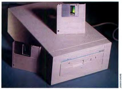
Pinnacle Micro's REO-130 takes erasable optical storage into the smaller 3½-inch disc format for the first time. The disc stores up to 133MB of data and will fit into a shirt pocket.
