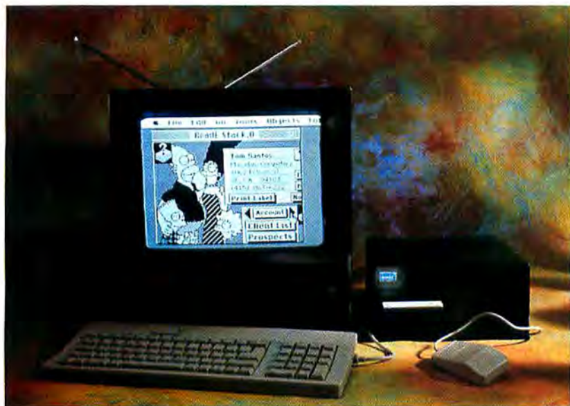
The Road E kit from Macadam Computer converts an SE or SE/30 into a transportable Mac. An optional NTSC driver hooks the Road E to a TV so you don't have to tote a monitor.
