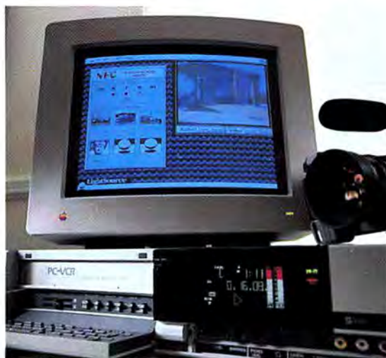
Light Source's MultiMedia Toolkit software lets the Mac control NEC's PC-VCR, a high-speed editing video recorder.
