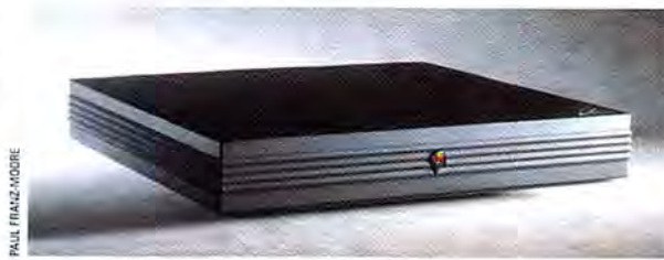
Pizza, Anyone? Both the Nextstation and the Nextstation Color CPUs reside in low-profile boxes that hold 68040 chips, 2.88MB floppy drives, and built-in networking.
