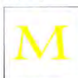
Trapping for Yellow on Magenta specified as Overprint.
