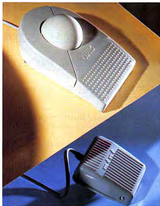
The MVP Foot Switch, an ergonomic option for Curtis's MVP Mouse trackball, acts as a fourth switch.
