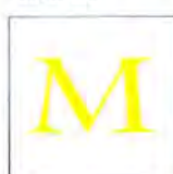
Trapping for Yellow on Magenta specified to choke .75 pt.
