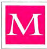
Trapping for Yellow on Magenta specified to spread .75 pt.
