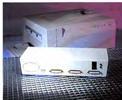
PageBlaster and its UltraScript software rasterize PostScript files into bitmaps for output on a non-PostScript printer (rear).
