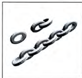
The chains were made by creating one link of the chain, then duplicating and rotating, and repeating the process until the chain was complete.
