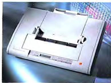
The Kodak Diconix Color 4 ink-jet printer uses four nonsmear inks that were specially formulated to blend together well.
