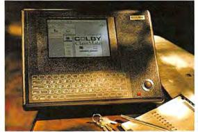
The Colby ClassMate, which has a pressure-sensitive membrane keyboard, is the lightest Mac portable to date.
