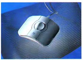
The Stingray Ergonomic Trackball was designed with a low profile so the user's wrist doesn't bend awkwardly.
