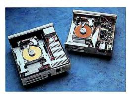
The drive on the left shows a well-shielded power supply, while the one on the right uses no shielding. Shielding is important because all power supplies generate electric and magnetic noise that can get into SCSI cabling and cause data-transmission errors.
