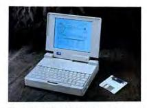
The Outbound Notebook System weighs only 6.5 pounds including an internal hard drive with a capacity of up to 60MB.
