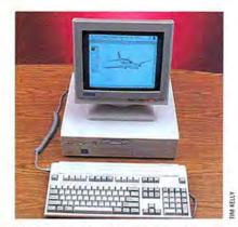
The BlueMaq Heat Seeker II includes an accelerated Mac SE system board, a monochrome monitor, and a display adapter.
