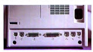
The back panel of the Macintosh Classic II includes (from left) a microphone jack; an ADB connector; a floppy drive port; a SCSI port; two serial ports; and a two-channel monophonic headphone jack.
