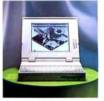
With a 60MB hard drive and 5MB of RAM, the Compaq LTE 386s/ 20 is a strong performer. Its display contrast was the highest, and its brightness among the best. The keyboard has firm, large keys. The LTE also offers a sliding door to cover the I/O ports.
