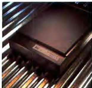
THE 6C OMNIMEDIA FROM XRS IS A 600-DPI FLATBED SCANNER FOR PAPER OR TRANSPARENCIES.
