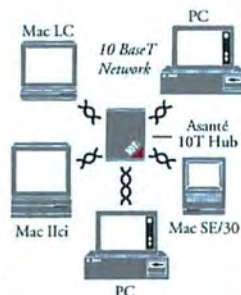
[ Asanté's 10T Hub/8 allows computers to be connected via inexpensive UTP media. ]
