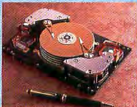
CONNER PERIPHERALS' CHINOOK SERIES OF HARD DRIVES HAVE TWO INDEPENDENT READ-WRITE HEADS FOR GREATER SPEED.
