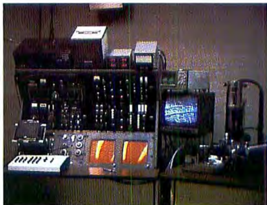
David Scharf's modified scanning electron microscope, or SEM. On the far right is the electron optical column. On the left is the console containing all the amplifiers and controls. The color processor is the keyboardlike object that sits on the left side of the console's desktop.
