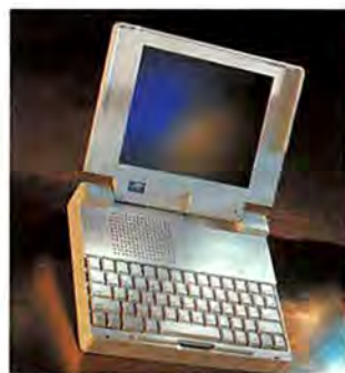
THE OUTBOUND NOTEBOOK SYSTEM 2030 HAS TWO MODELS: ONE WITH A 25MHZ 68030, THE OTHER WITH A 33MHZ 68030.
