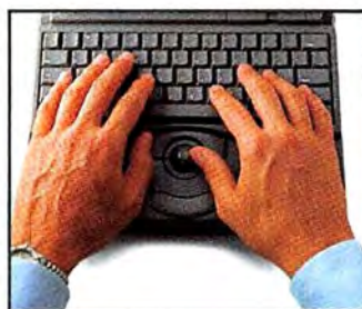
An integrated trackball and palm rests make the PowerBook keyboard extraordinarily comfortable for both left- and right-handed people to use.
