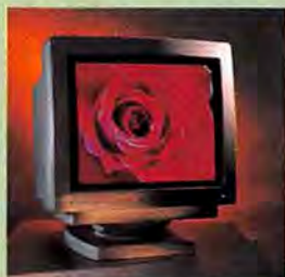
THE RASTEROPS SWEET SIXTEEN SYSTEM COMBINES A 16-INCH MONITOR WITH A 24-BIT GRAPHICS ADAPTER BOARD.
