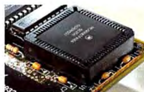
[ The MacCon+ LC has an on-board socket for adding an optional Motorola 68882 math co-processor. ]
