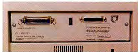
NTR Printer Ports The NTR provides more flexible attachment to computers. From left to right, the Centronics parallel port, thumb-wheel setting for specifying emulation modes to ports, serial port, and LocalTalk port.
