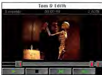
Captured Live ScreenPlay, the program that comes with SuperMac's VideoSpigot video-capture board, lets you view a clip as it's being recorded, set the in and out points, and save it as a QuickTime movie.
