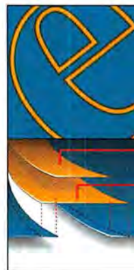
Top stroke knocks out Bottom stroke is wider and over-prints
