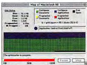
THE NEW MACTOOLS HAS A GRAPHIC DISPLAY SHOWING A DISK'S FRAGMENTATION.
