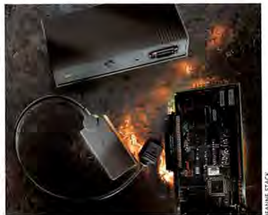
Ethernet Options Clockwise from lower left: Apple's Ethernet Twisted-Pair Transceiver, Asanté's EN/SC SCSI-to-Ethernet Adapter, and Shiva's EtherPort II NuBus Card
