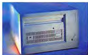
THE RICOH HYPERSPACE SHUTTLE IS AN ERASABLE OPTICAL DRIVE THAT CAN CHANGE UP TO FIVE 650MB CARTRIDGES.
