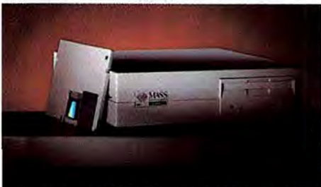
A Mass Micro technology breakthrough: DataPak MO/128's 3½-inch removable, rewritable optical storage.
