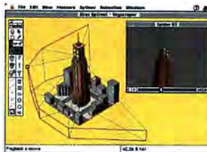
ALIAS UPFRONT 2.0 WITH SPIDER VISION—A SERIES OF LINES DESCRIBING THE PATH OF A FLY-THROUGH.
