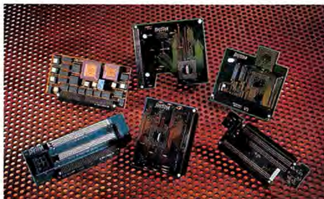
Rather than create a different board for each type of Mac Processor Direct Slot, DayStar Digital uses one common board (upper left) and offers adapters to connect it to each type of Mac PDS.
