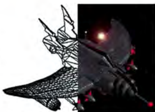
STRATAVISION'S SKIN MODELER CAN WRAP A SURFACE OVER MANY DIFFERENT-SHAPED RIBS.
