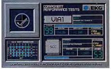
MacEKG tests individual hardware components to seek out possible faults — before they become major problems. The VIA (Versatile Interface Adaptor) chips handle all user input like the mouse and keyboard. A faulty VIA can cause inconsistent cursor movement, and if allowed to get worse, complete system shutdown,
