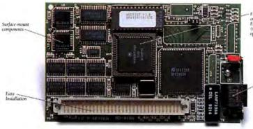
FPU Socket included on all LC and IIsi Etherl AN cards (shown with (shown with optional FPU)
