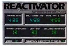
For intermittent failures, you need to Reactivator. If continually tests, powers down and retests until the problem surfaces. This is a heaven-sent tool for anyone trying to find heat-related problems.
