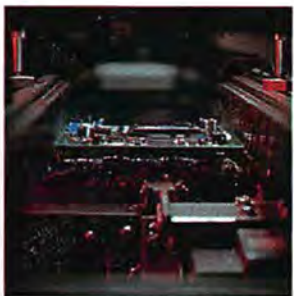
CONNECTING CIRCUITS By dipping protruding pins in a 237°C solder bath, manufacturers secure sockets and other parts to the logic board circuitry. Most chips don't have pins poking through holes in the logic board; they mount directly on its surface.
