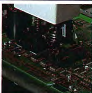
PLACING PARTS A robot rapidly picks up a chip, scans it for damage, and places it with 1/1000-inch accuracy on the logic board.
