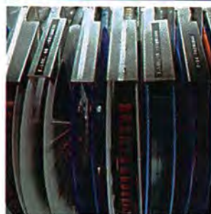
STOCKING SUPPLIES Chips arrive wound around reels on 35mm strips or arrayed in trays, pre-tested and ready for use.
