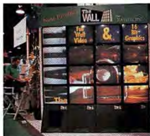
RASTEROPS' WALL CAN HAVE UP TO 16 MONITORS STACKED 4 HIGH AND CONTROLLED BY A MAC.
