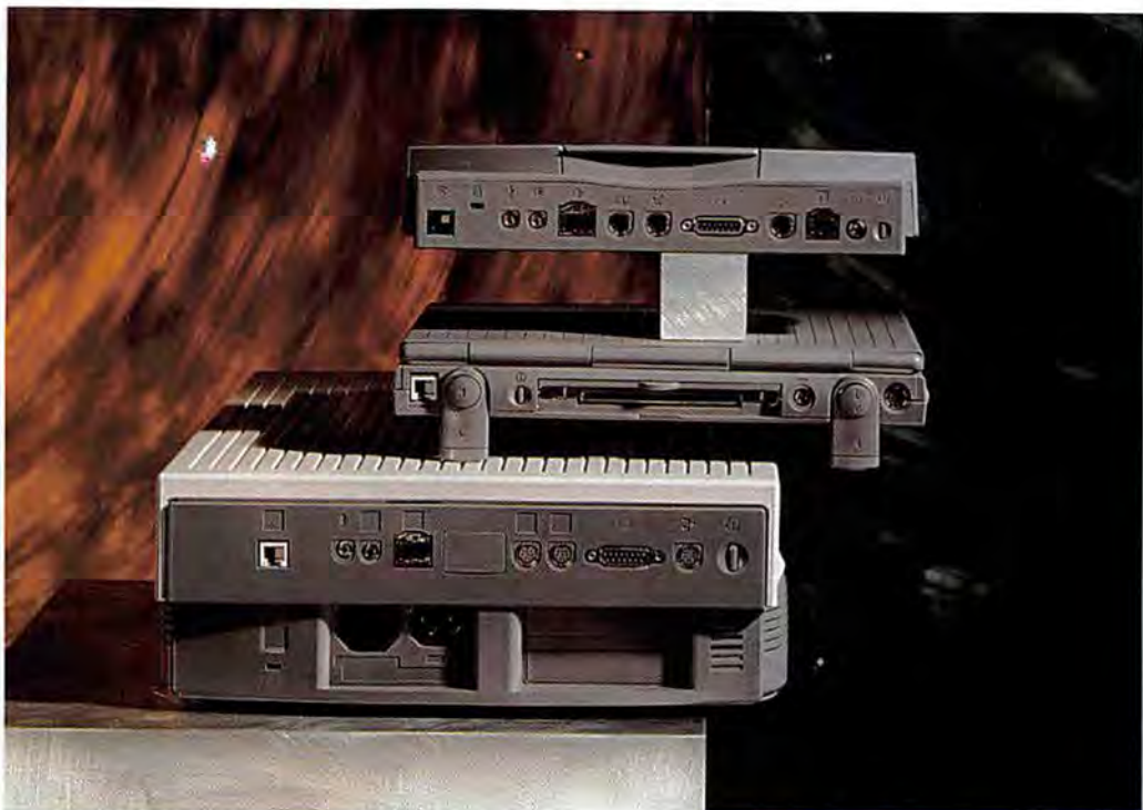
Comparing Ports Stacked up here in order are the Duo MiniDock (top), PowerBook Duo 230, and the Duo Dock. As you move from top to bottom of this photo, you increase your possible connections to the outside world as well as your expansion options.
